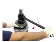
Use TORQUE TESTING NUT and WRENCH to tight at correct torque (clockwise) (Step 9)
