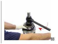
Use TORQUE WRENCH WITH INSERT to tight at correct torque (clockwise)
