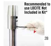
Remove metallic filter grid from INTERCONNECTOR
