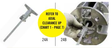
Pull out SHAFT using DEPTH TOOL
