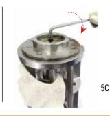
6 Set down FIXTURE SEAT and tighten using HEXAGONAL ALLEN TOOL FIXST (clockwise)
