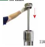
Use WRENCH FOR IMPELLER NUT TOOL to tighten (clockwise)
