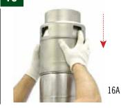
Make sure bolts on discharge are aligned with bolts in INTERCONNECTOR
