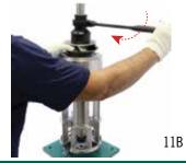
**Use TORQUE TESTING NUT and** WRENCH to tight at correct torque (clockwise) (Step 9)
